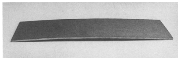
Figure 1 Typical arcing of a sheet specimen after shot peening.
